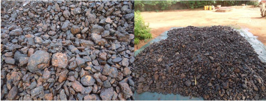
**Figure 1: High grade manganese produced by screening on site at Nayega**
